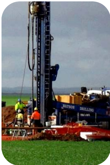
Adelaide Plains drilling operations utilising Watson Drilling diamond core rig.
